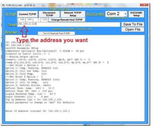
Figure 3-32, Enter new IP address
