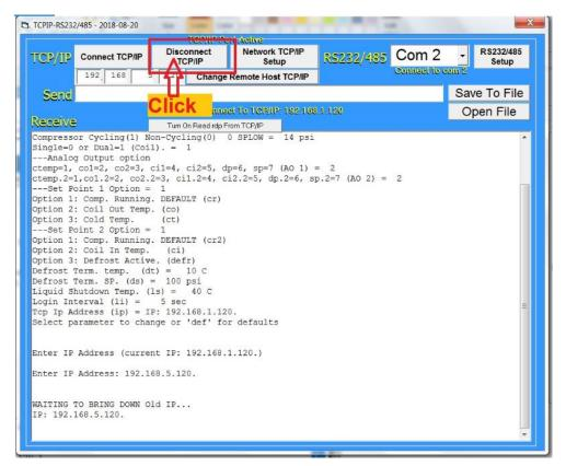
Figure 3-33, Disconnect TCP/IP
