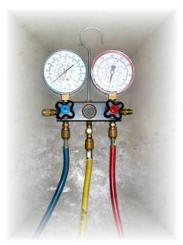
Figure 3-8, Refrigerant Manifold
