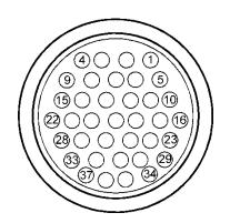
Figure 3-13, 37-Way Amphenol™ Connector, Front view
