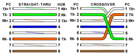
Figure 3-14, Ethernet cable (crossed)
