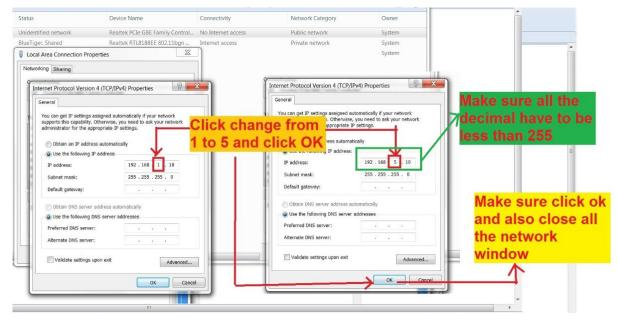
Figure 3-34, Change Remote Host IP address
