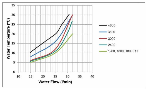
Figure 3-4, Water flow Requirements
