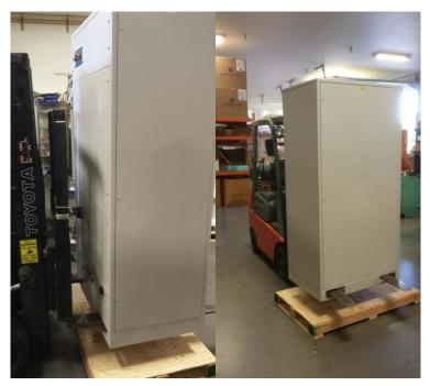
Figure 3-1, Removing Unit from Transportation Pallet
