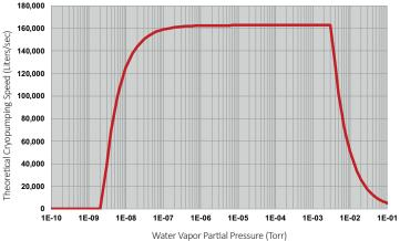
Single-circuit model; 2.4m refrigerant line; typical cryocoil surface area only; larger cryocoils will give greater pumping speeds and can be used in some applications; 25°C chamber temperature in line of sight with cryocoil; 60Hz; 25- 28°C cooling water.
