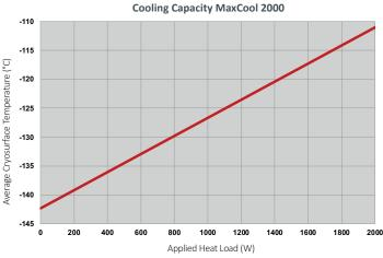
Single-circuit model; temperature shown is average of inlet and outlet temperature using typical cryocoil size; temperature difference between inlet and outlet at maximum load is typically 20°C; end point of curve is maximum load; performance at 50Hz can be 3-5°C warmer than 60Hz performance shown; 25-28°C cooling water.
